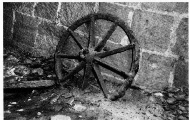
A CM&GIR wagon wheel, the most complete of four such wheels found at the base of the flooded slope shaft in Merstham quarry. Photo: the late John Maneely
